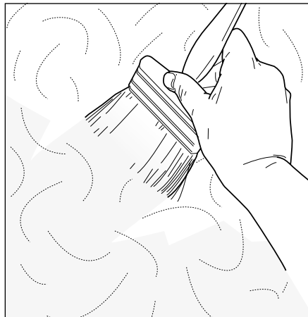
Gently brush on penetrating fluid, or dampen and loosen the coating with steam
