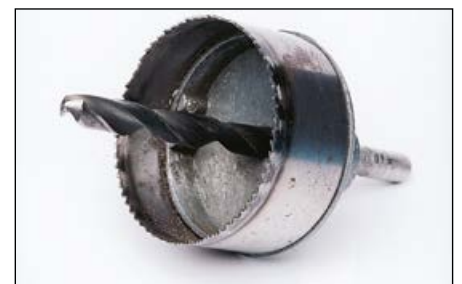
Use a hole cutter for holes greater than 20 mm
